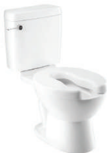
SC6657 Forall 40 Dimension 430 x 780 x 775 mm. Type / Shape Two Piece toilet / Elongate Pipe S-trap 305 mm. Water system Wash down 4.5 Liters
