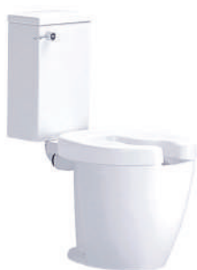
SC6652 Forall Dimension 420 x 740 x 925 mm. Type / Shape Two Piece toilet / Elongate Pipe S-trap 305 mm. Water system Wash down 3.8 Liters
