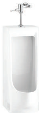
C31207 Hercules Dimension 325 x 415 x 1000 mm. Type / Shape Floor Stand Pipe P-Trap, Rough-in 200 mm. Water system Top inlet
