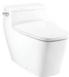
C101907 Hercules Curve Dimension 450 x 745 x 600 mm. Type / Shape One Piece toilet / Rectangle Pipe S-trap 305 mm. Water system V-Silent 4.8 Liters
