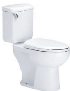
C1302 Sydney 45 Dimension 390 x 790 x 840 mm. Type / Shape Two Piece toilet / Elongate Pipe S-trap 305 mm. Water system Siphonjet 6 Liters
