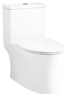
C105607 Vista Dimension 400 x 710 x 755 mm. Type / Shape One Piece toilet / Rectangle Pipe S-trap 305 mm. Water system Siphonjet 4.8 Liters
