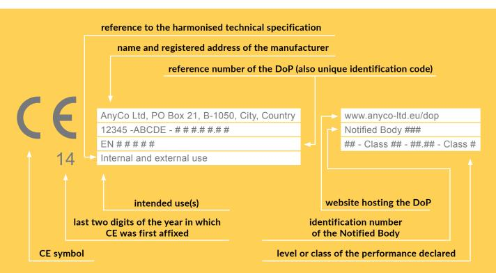
EXAMPLE: Bulk aggregates are usually CE marked in the accompanying documents, usually together with the despatch note provided by the manufacturer.
